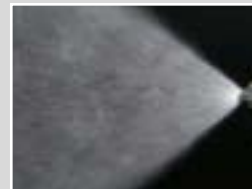
Pattern collapse with PermaFlo™ 830 pump
