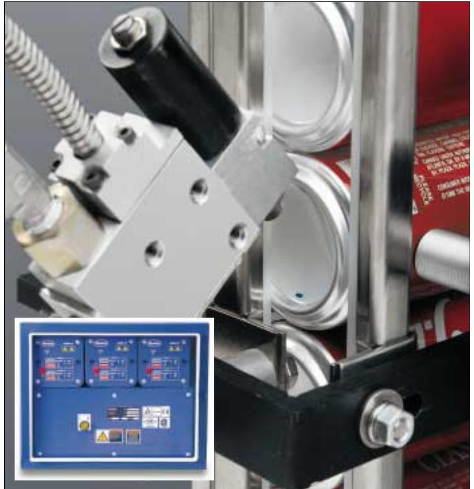
Ink-Dot I.D. system controller with enhanced Series II driver.
