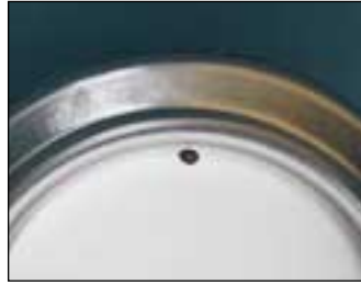
A different color dot is applied by each spray machine for immediate identification of the malfunctioning spray machine.
