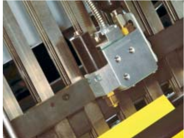
Compact electric hot melt dispensing guns deliver precise, consistent adhesive application.
