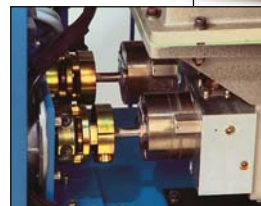
Pump shut-off valve and single-tool removal provide quick, easy pump replacement
