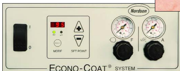
The Econo-Coat gun controller features easy selection/adjustment of kV and micro-amp setpoints.
