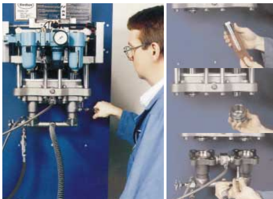
The plungers and packing glands can be easily replaced on-line in 20 minutes.
