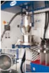
Optional feed center allows for fully automatic powder-to-gun delivery and recovery with sieving, and return of the powder to suppliers' boxes for maximum powder usage and minimal material loss.
