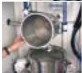
Optional feed center allows for fully automatic powder-to-gun delivery and recovery with sieving, and return of the powder to suppliers' boxes for maximum powder usage and minimal material loss.
