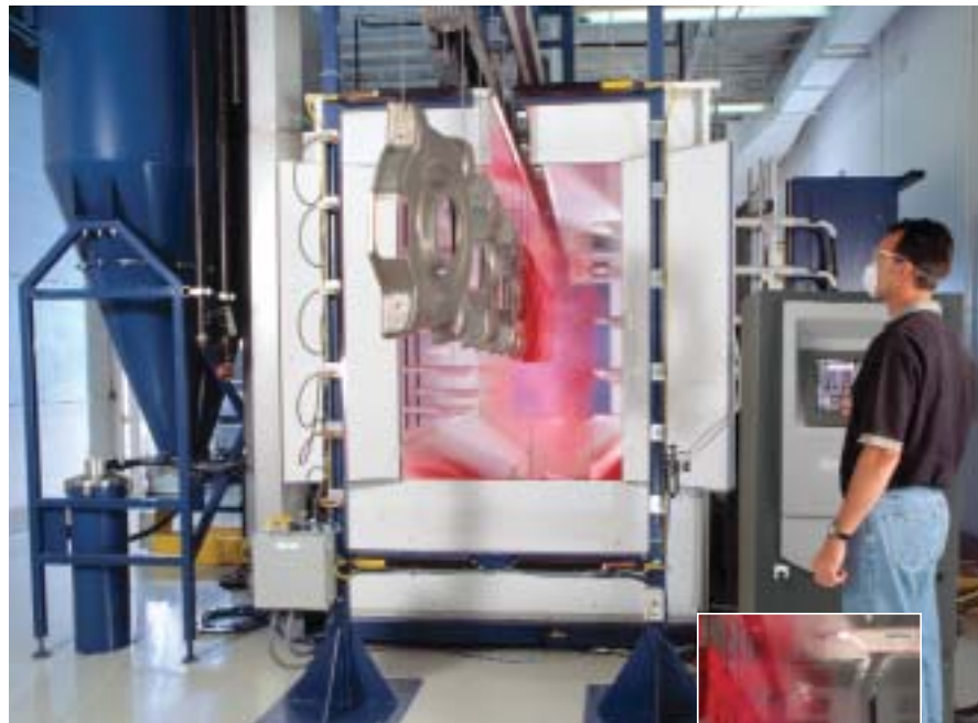
The ColorMax booth has no inlet ductwork that must be inspected and cleaned for no doubt that the system is clean.
