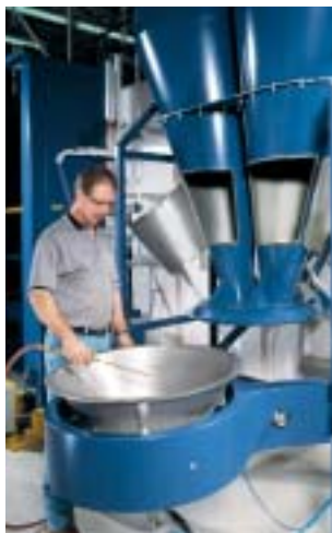
Twin cyclones facilitate complete cleaning without cross-contamination.
