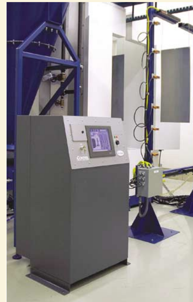
Figure 5. Photoeyes connect to the control system to trigger spray guns on/off.
