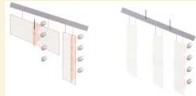
Figure 4. Large gaps between and around parts of differing shapes and sizes are common.
