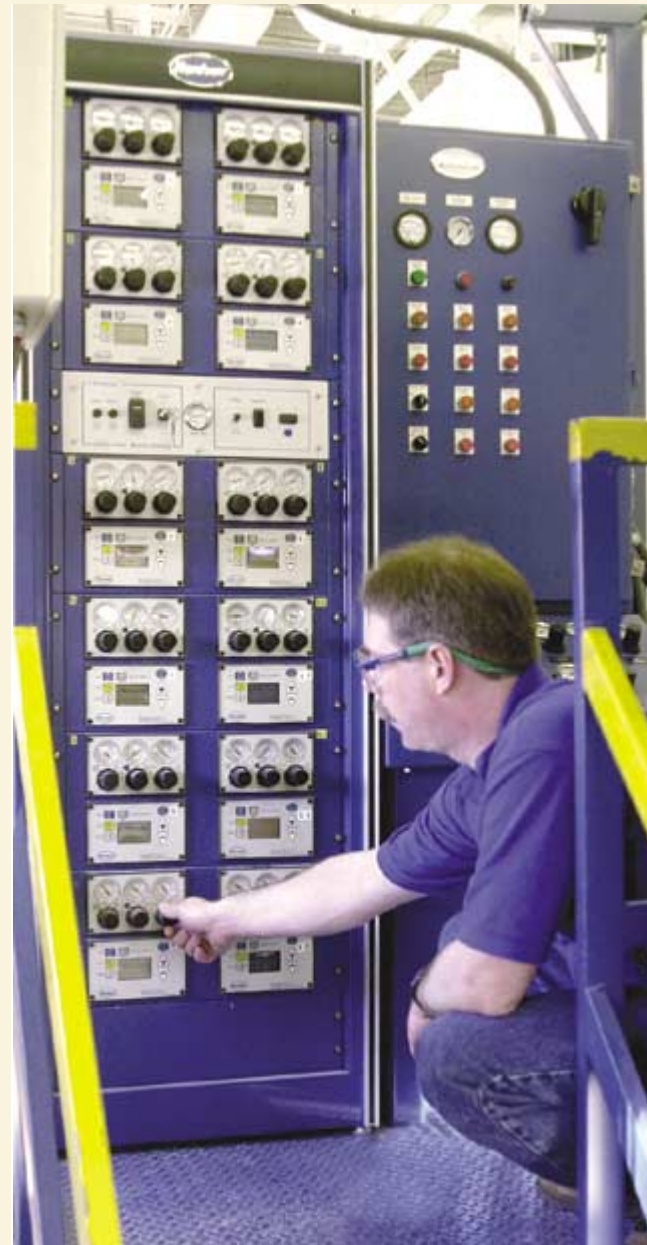
Figure 1. Manually adjusting traditional powder regulators has some inherent problems with accuracy and consistency.
